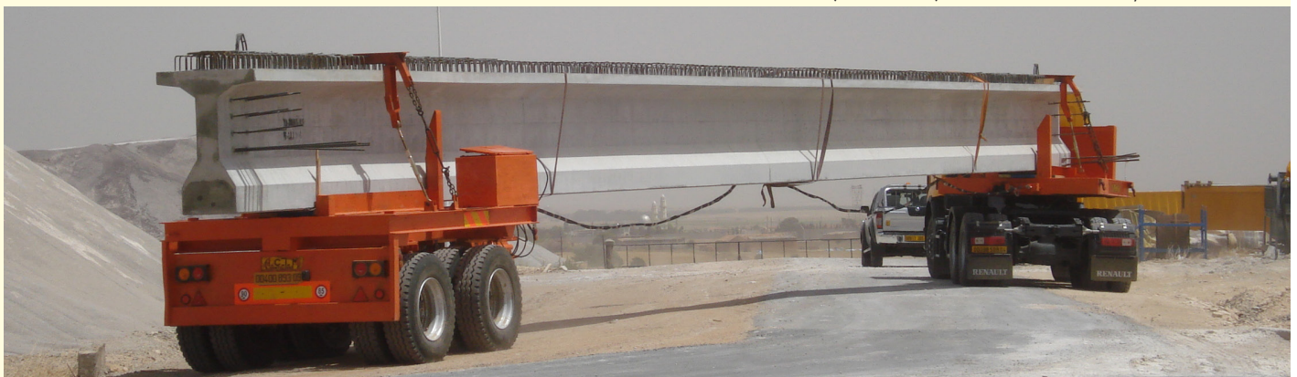
Gambar (Illustration) 02. Balok Jembatan / I Girder
