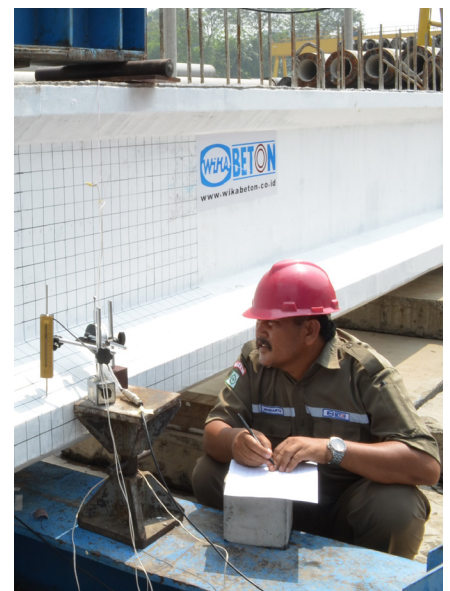
Gambar (Illustration) 09. Uji Beban Girder/ Girder loading test
