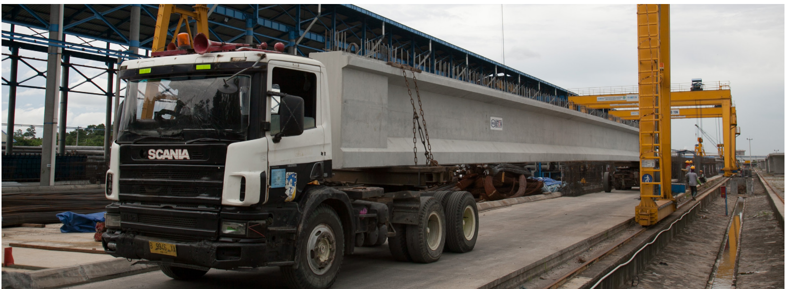
Gambar (Illustration) 06. Distribusi Balok Jembatan/ Distribution of Girder
