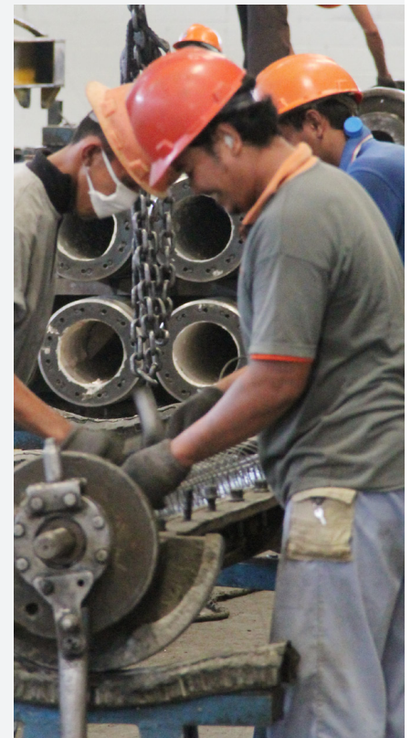
Gambar (Illustration) 22. Proses pemasangan cetakan/ Mould installation process
